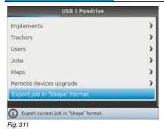
Allows to memorize job data onto a map, saving it onto the pendrive. Data in the file can be displayed on a Personal Computer with a "Shape" file viewer (.shp).
