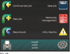
After the software version, Bravo 400S displays the Select User prompt (Fig. 37) Press F4 or F6 to move across the available items, then press  $\square K$  to confirm your selection. At this point, Bravo 400S displays the "Home" screen (Fig. 38).
