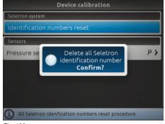
Allows to reset the identification numbers of all saved Seletrons, before repeating the pairing procedure (chap. 11).
