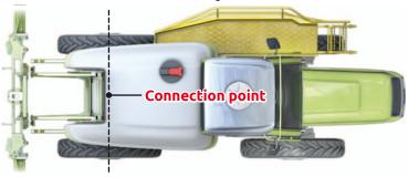
THE CONNECTION POINT OF A SELF-PROPELLED MACHINE **COINCIDES WITH THE REAR AXLE** OF THE VEHICLE.
