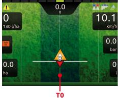
When this function is used, Bravo 400S deletes the previous reference track **T0** (if present), and prompts the operator to save two NEW points **A** and **B** on the field, which create a NEW reference track.
