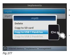
Allows to copy data from Bravo 400S internal memory onto a pendrive.
