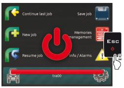
Keep ESC key pressed until Bravo 400S is switched off.
