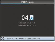
"PDOP" and "HDOP" are parameters that depend on the position and number of satellites in space that affect the positional precision of the system (longitude and latitude); the lower the value, the higher is the driving precision.
