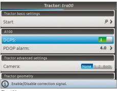
Allows to enable / disable the DGPS (SBAS) differential correction function
