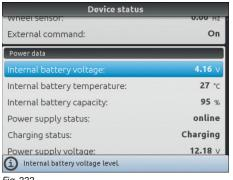
Bravo 400S checks the status of the power supply.
